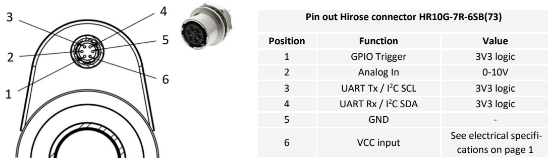
Figure 3: Electrical connections of ECC-1C featuring (female) Hirose connector.
